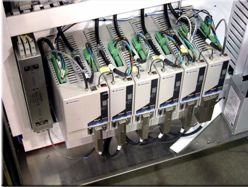
*Figure 6.28: Servo Controllers*
