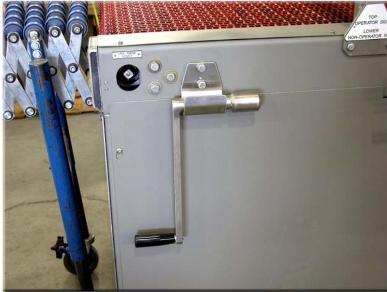
*Figure 6.18: Tunnel Chain Handle*
