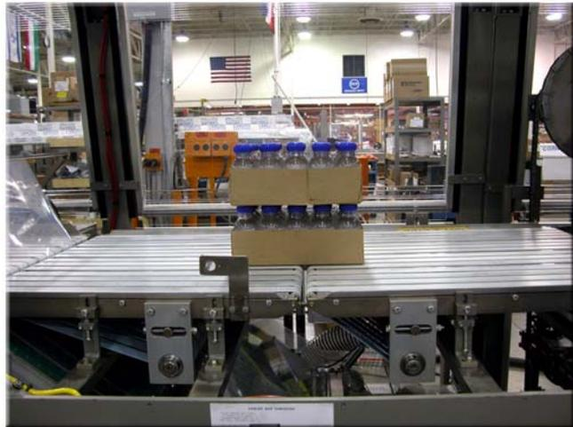
*Figure 5.5: Product on the Wrapper Infeed Conveyor*
