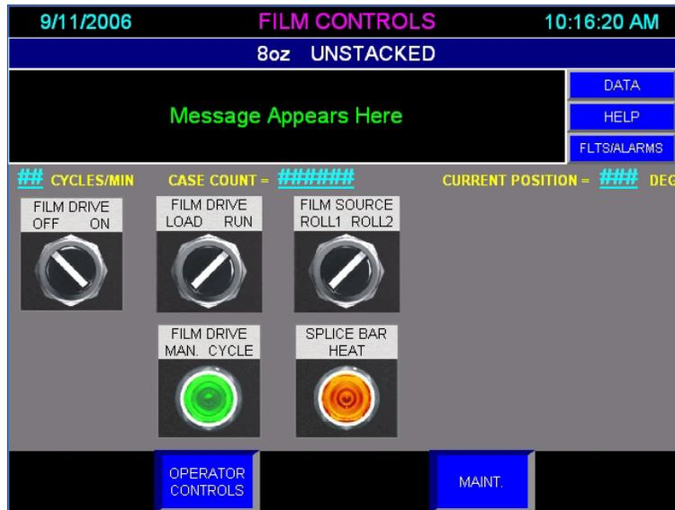
Figure 8.2: Film Controls Screen
