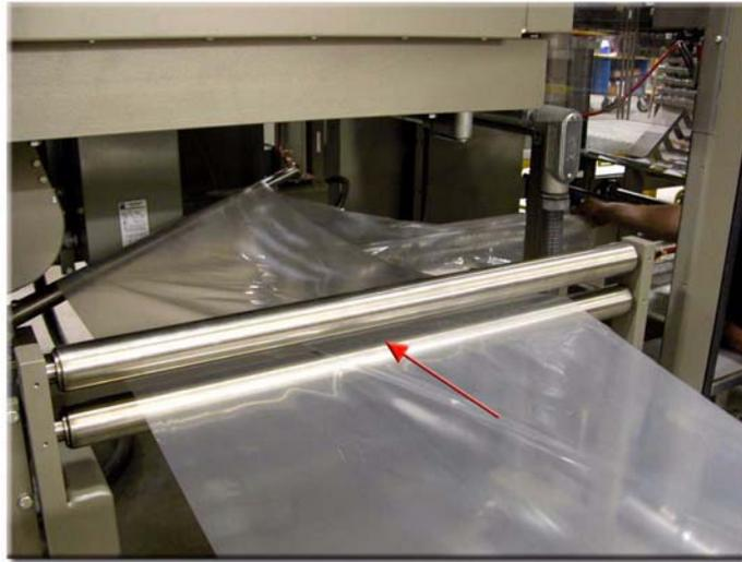
*Figure 3.32: First Guide Rollers*
