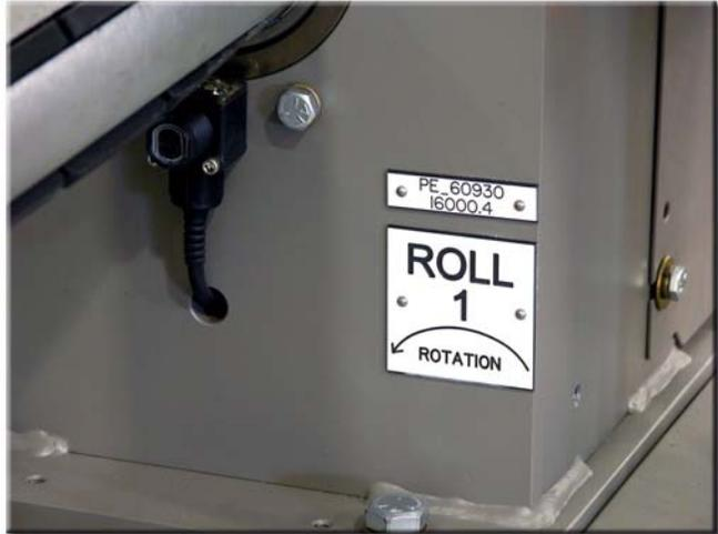
Figure 5.16: Low Empty Film Roll 1 Photoeye
