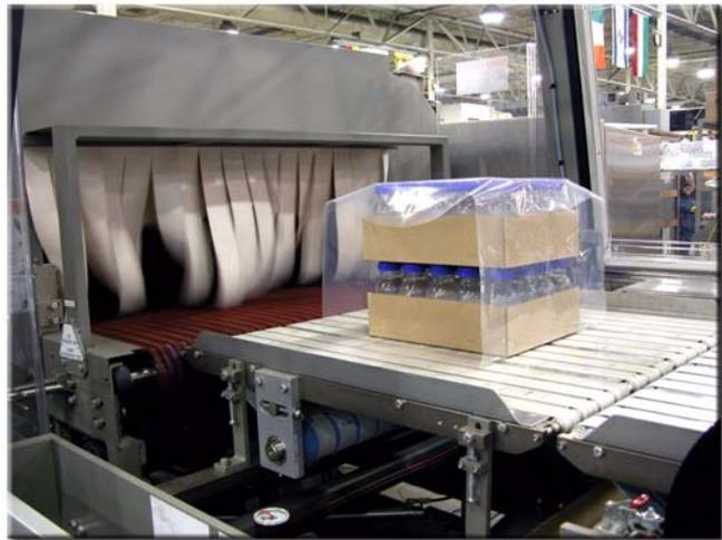
*Figure 5.7: Product on Wrapper Discharge Conveyor*
