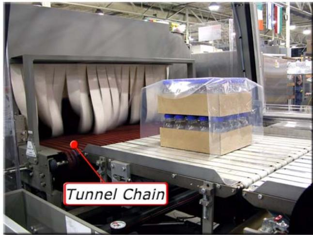
Figure 5.17: Tunnel Conveyor Chain
