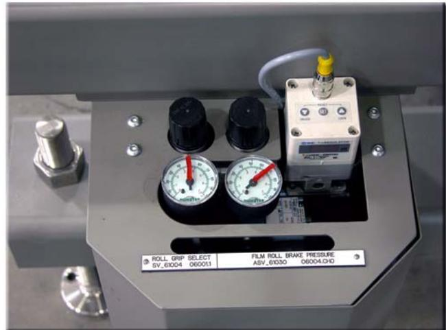
*Figure 5.14: Film Roll Brake Pressure Regulator Valve*
