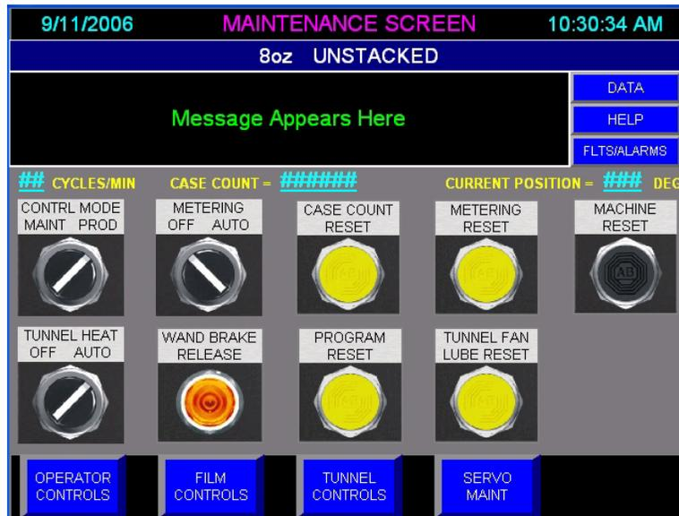
The **Wand Brake Release** pushbutton releases the wrapper wand when safety circuit(s) are open, allowing the wand to move freely.
