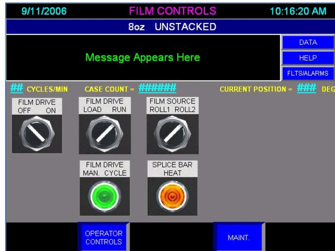
*Figure 3.52: Film Controls Screen*
