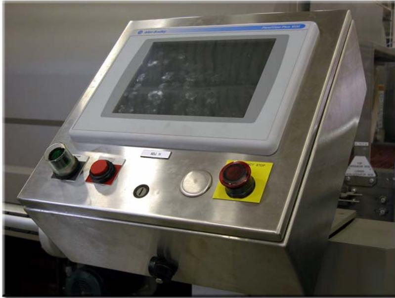
*Figure 3.1: Main Control Panel*
