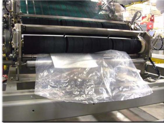
*Figure 3.39: Card in Pinch Roller*
