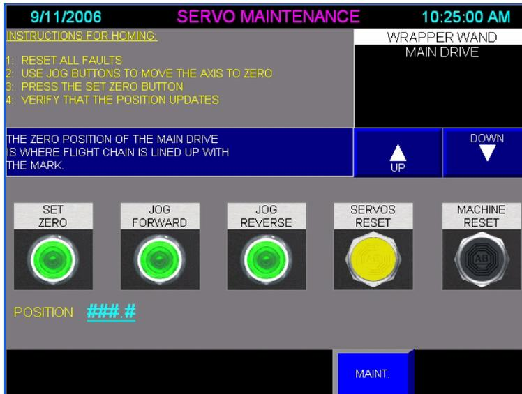
*Figure 8.4: Servo Maintenance Screen*
