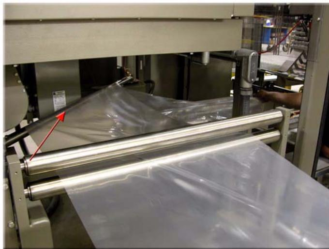
*Figure 3.33: 45 Degree Angle Bar*
