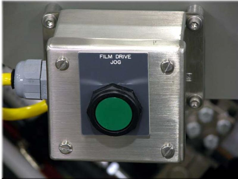
*Figure 3.26: Film Drive Jog Pushbutton*
