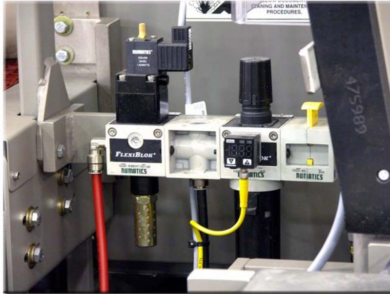
*Figure 1.2: Air Pressure Monitor*
