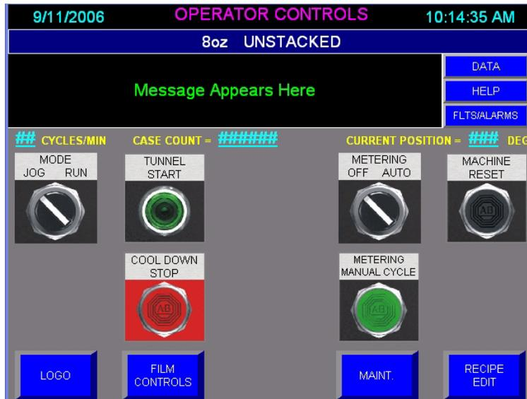
The **Cool Down Stop** pushbutton provides a sequenced shutdown to the tunnel. The heaters shut down first while the blower fan and belts continue to run until the tunnel has cooled sufficiently.
