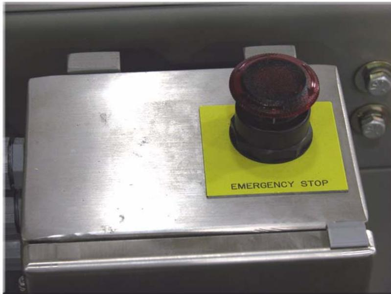
Figure 3.27: Auxiliary Emergency Stop Pushbutton
