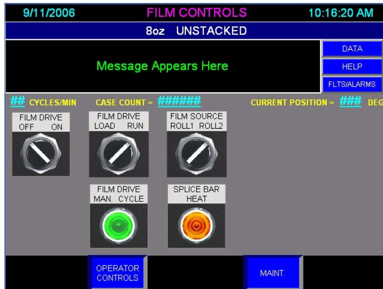
The **Film Drive Load/Run** selector switch, placed in the *Load* position, removes the brake tension from the film rolls. This action causes the rolls to be free-rolling which aids in initial threading and allows the use of the Film Drive Jog pushbutton. The selector switch is placed in the *Run* position for machine operation.
